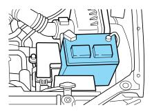
However, for severe usage or in high temperature climates, check the battery electrolyte level. Refer to the Scheduled Maintenance Guide for the service interval schedules.
